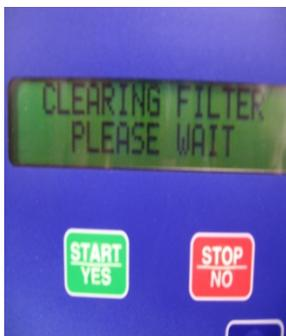
34700-2K – Press the START/YES button a second time to start the filter/dryer clearing process.
